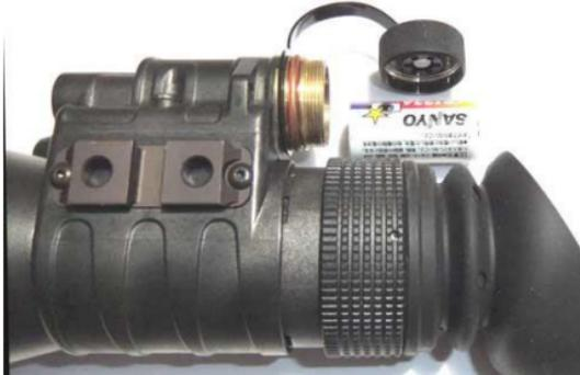
When the battery becomes discharged, a “yellow” low battery indicator light will be visible in the eyepiece. Unit is still safe to use for several hours, however the battery should be replaced as soon as practical.
